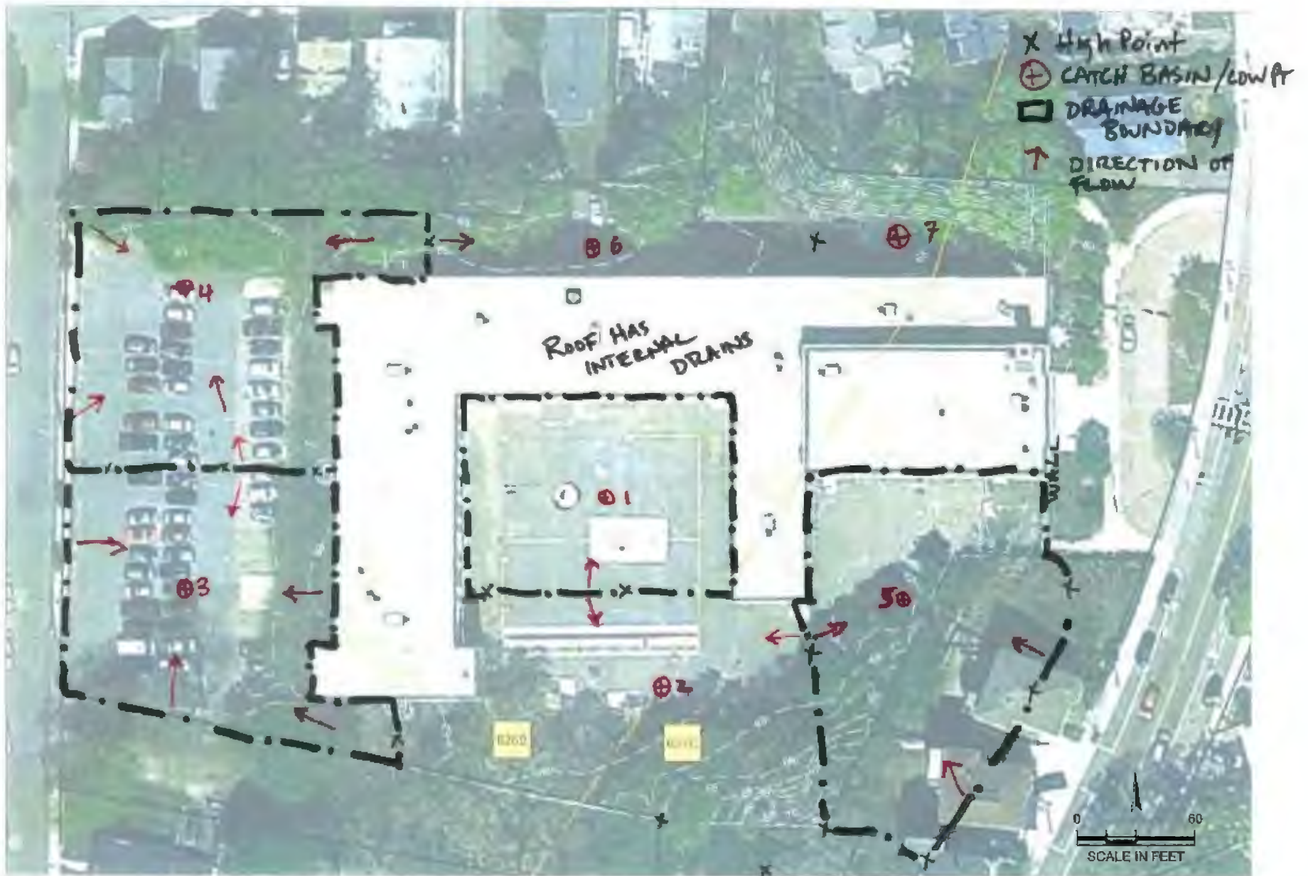
Figure 2. Field sketch of catch basins and drainage boundaries (THIS NEEDS TO BE TO SCALE FOR STUDENT USE)
