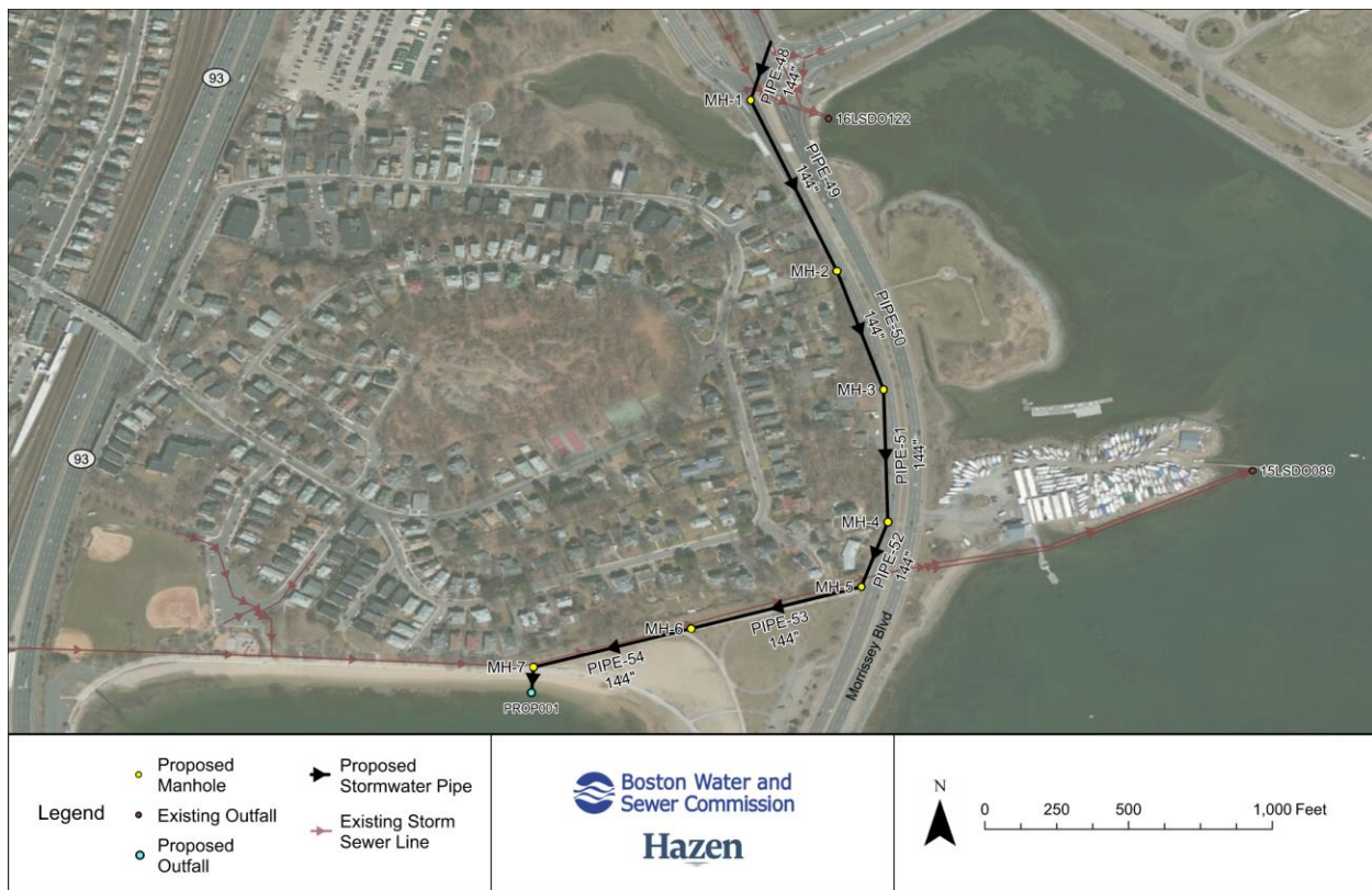
Figure 5-52: Outfall 16LSDO122 Diversion to Dorchester Bay Basin
