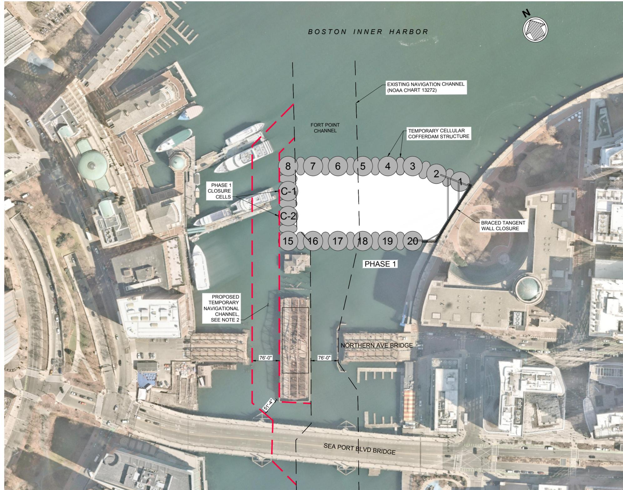
**A1** PLAN - STORM SURGE BARRIER - SUBMERGED AXIS FLAP GATE ALTERNATE - PHASE 1
