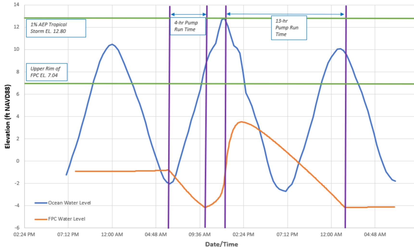
For the purpose of this evaluation, it was assumed that SSB gates were closed at low tide before the storm event and that the pumps were run to draw down the water level from the projected 2070 MLW elevation to the current MLW elevation to maximize storage. It was further assumed that gates remained closed throughout the storm event. During an actual storm event it may be possible to open the SSB gates when the exterior tide level drops below the water level in the basin.
