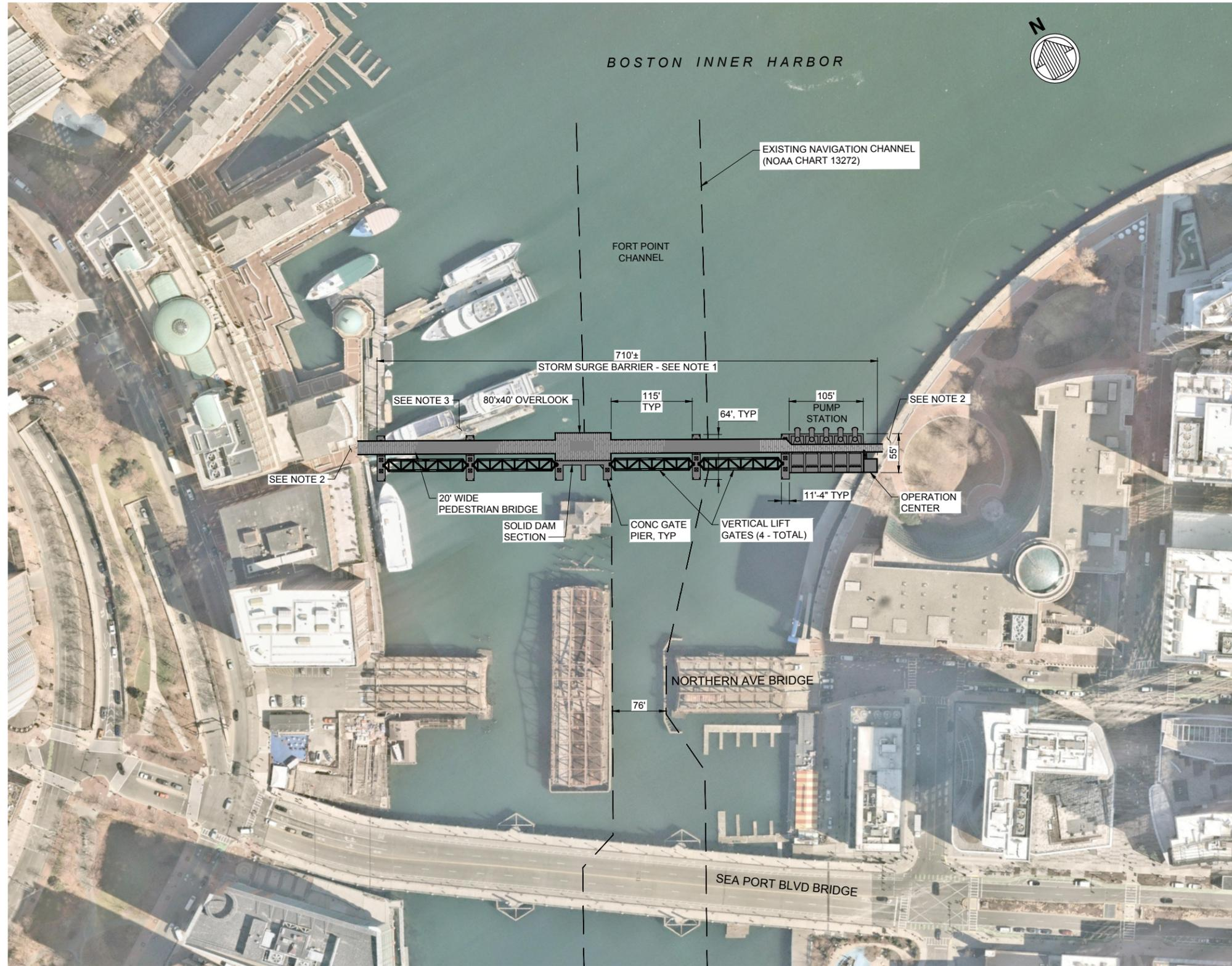
**A1** PLAN - STORM SURGE BARRIER - VERTICAL LIFT GATE ALTERNATE
