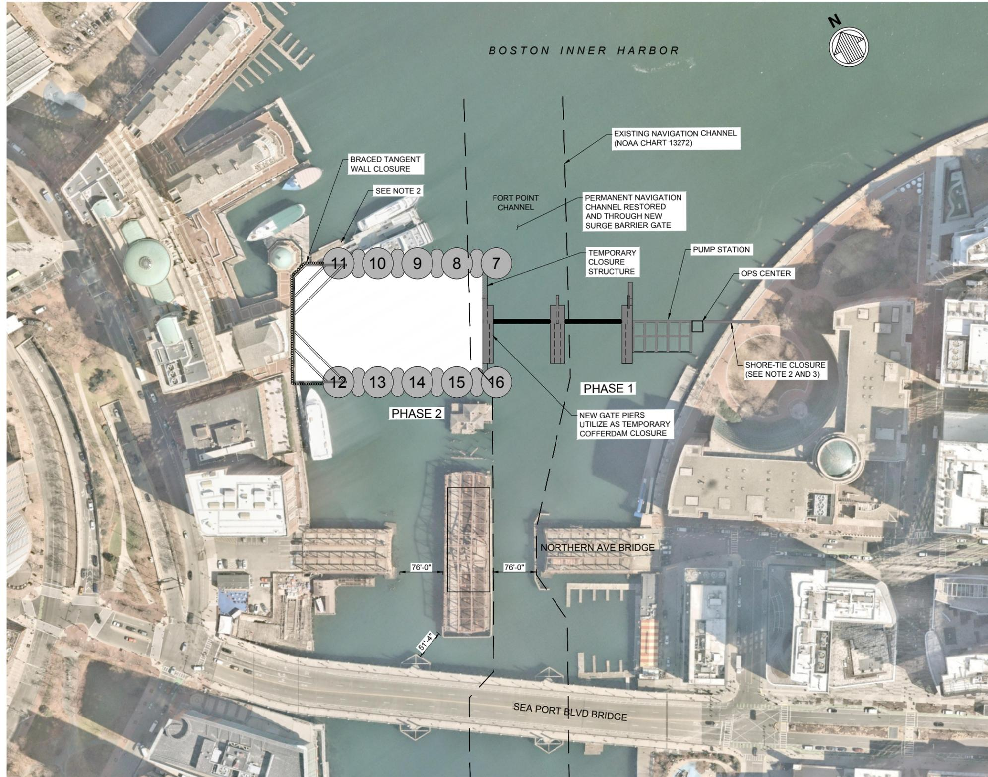
**A1** PLAN - STORM SURGE BARRIER - SUBMERGED AXIS FLAP GATE ALTERNATE - PHASE 2
