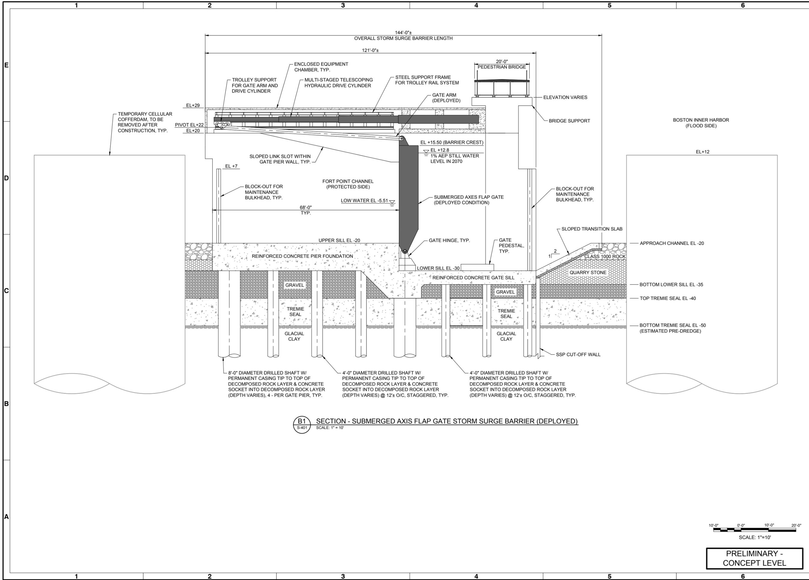
**B1** SECTION - SUBMERGED AXIS FLAP GATE STORM SURGE BARRIER (DEPLOYED)
