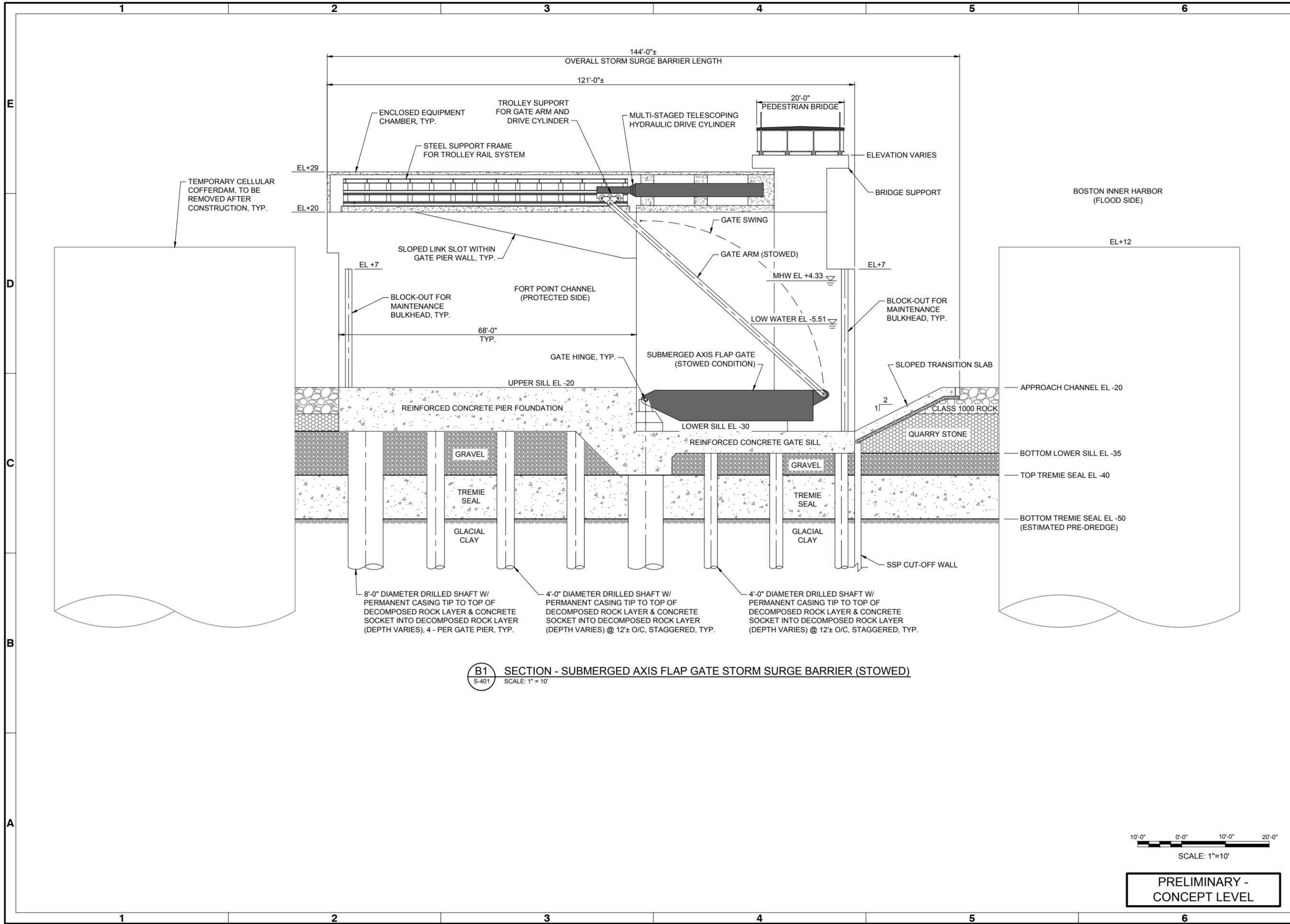
**B1** SECTION - SUBMERGED AXIS FLAP GATE STORM SURGE BARRIER (STOWED)
