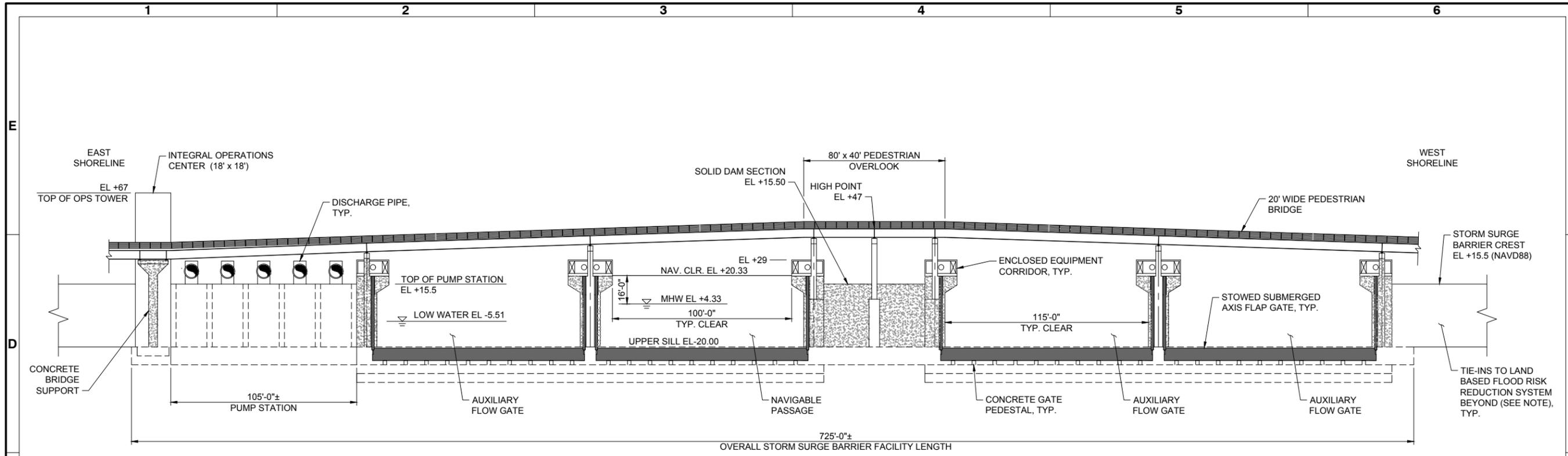
**C1** ELEVATION - SUBMERGED AXIS FLAP GATE STORM SURGE BARRIER - LOOKING TOWARDS FPC (GATES IN STOWED POSITION)
