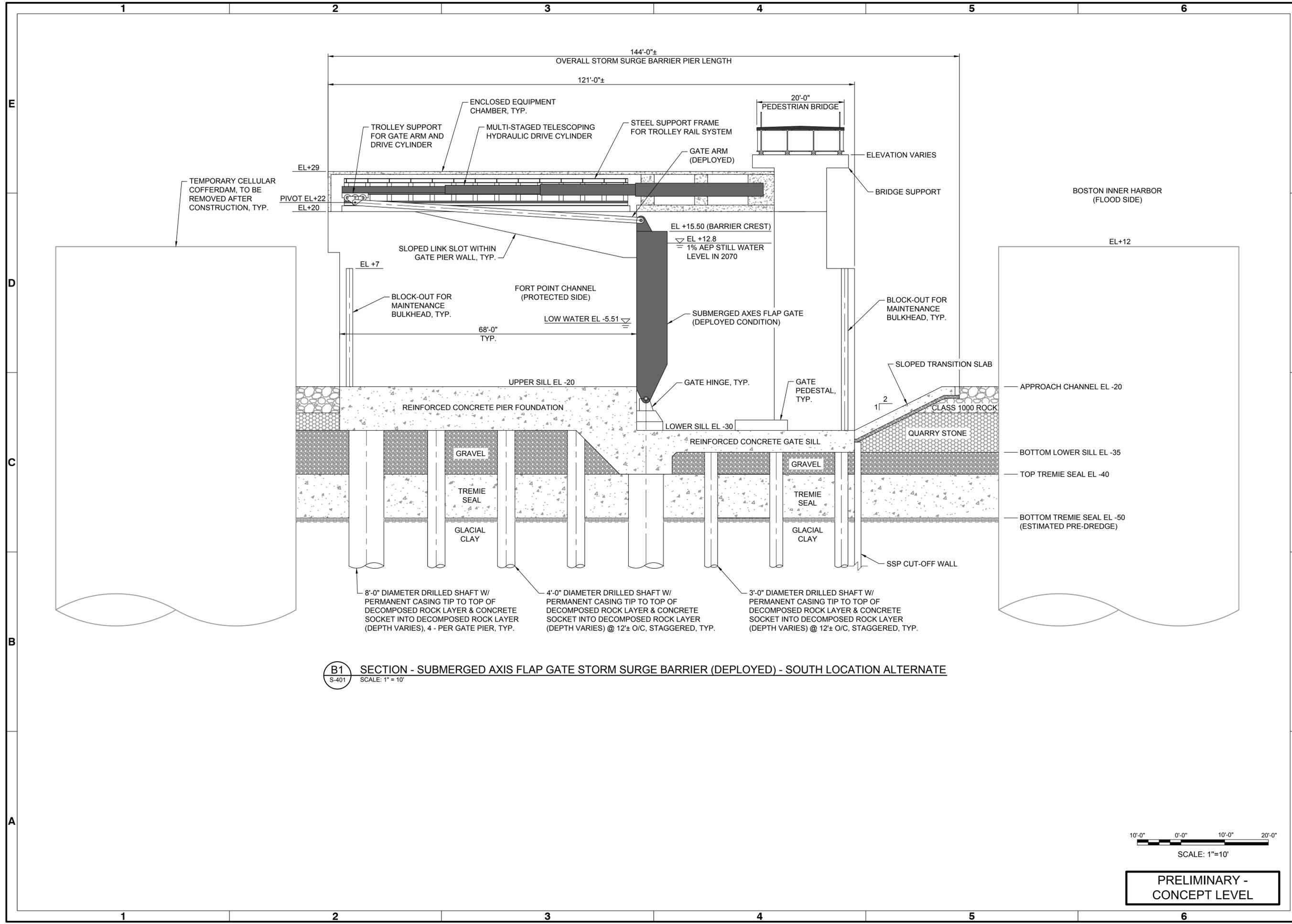
**B1** SECTION - SUBMERGED AXIS FLAP GATE STORM SURGE BARRIER (DEPLOYED) - SOUTH LOCATION ALTERNATE
