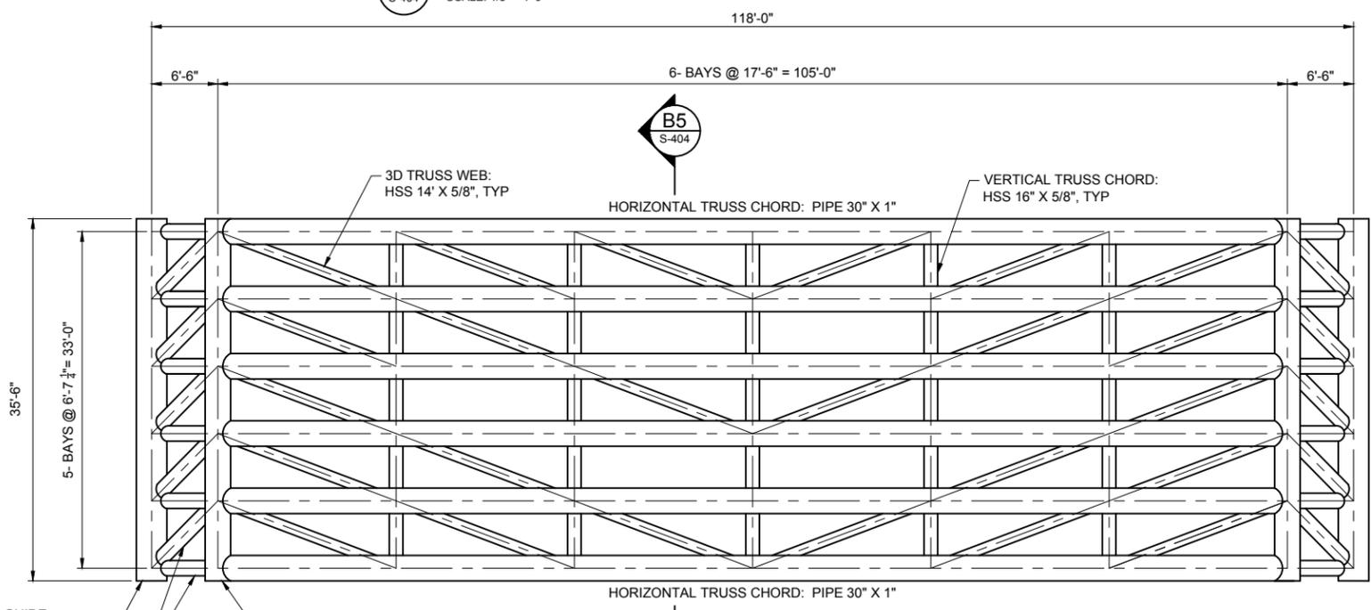
**B1** ELEVATION - VERTICAL LIFT GATE
