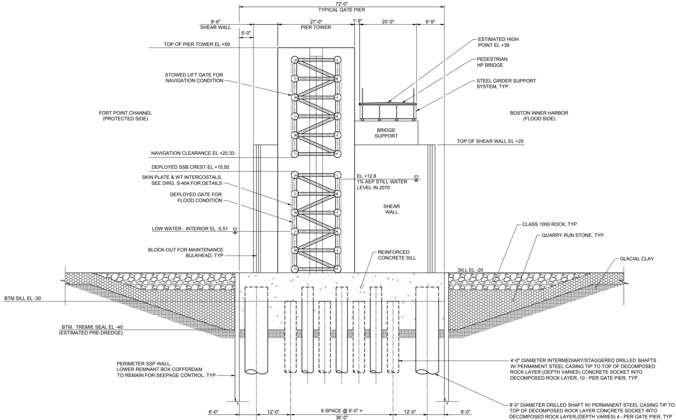
**B1** SECTION - VERTICAL LIFT GATE PIER
