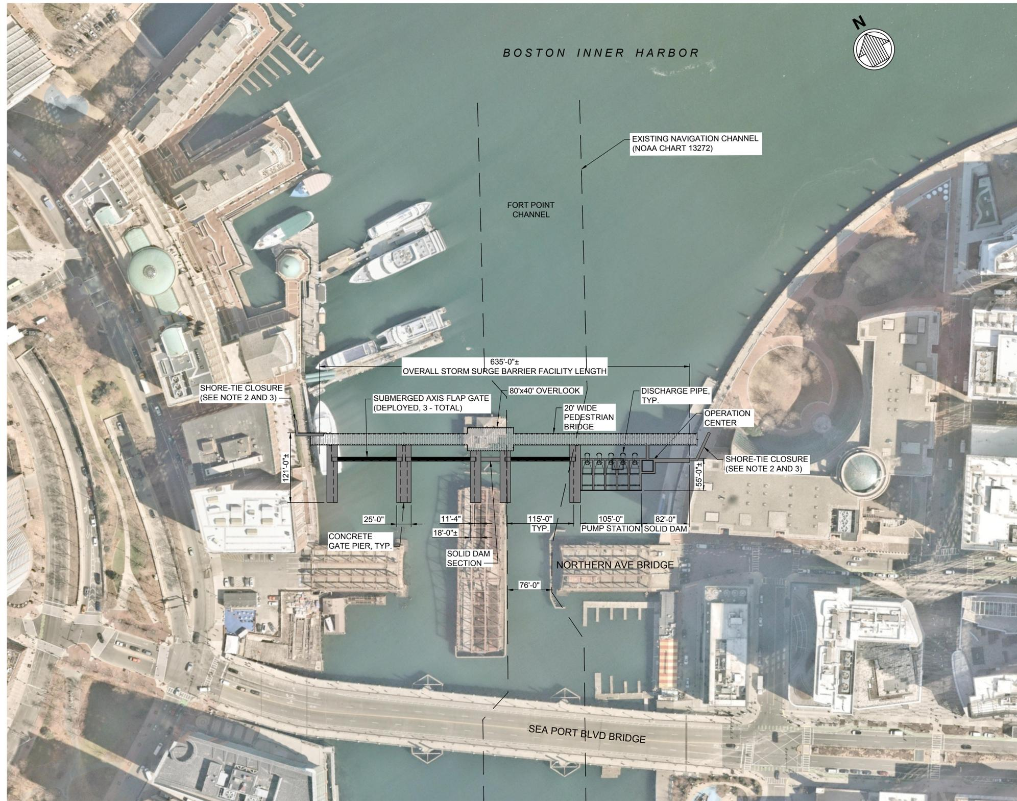
**A1** PLAN - STORM SURGE BARRIER - SUBMERGED AXIS FLAP GATE - SOUTH LOCATION ALTERNATE
