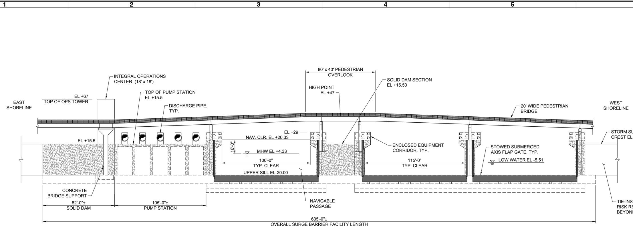
**C1** ELEVATION - SUBMERGED AXIS FLAP GATE STORM SURGE BARRIER - SOUTH LOCATION ALTERNATE - LOOKING TOWARDS FPC (GATES IN STOWED POSITION)
